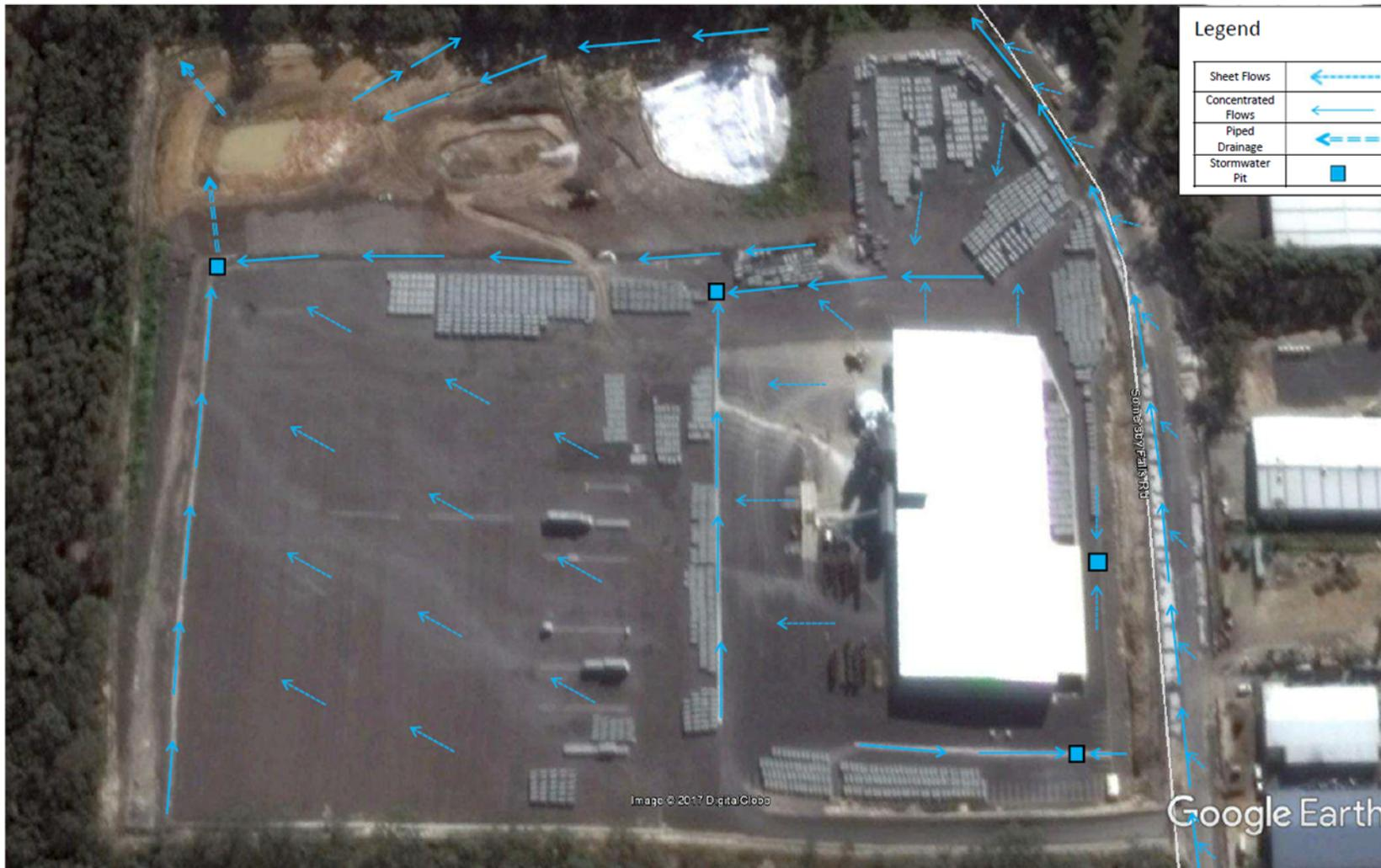
Figure - Overland Drainage Path Diagram
